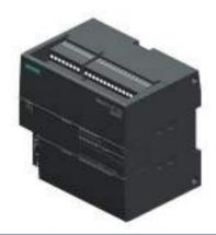
SIMATIC S7-200 SMART CPU CR30s, COMPACT CPU, AC/DC/RELAY, ONBOARD I/O: 18 DI 24V DC; 12DO RELAY 2A; POWER SUPPLY: AC, 85 - 264 V AC AT 47 - 63 HZ, PROGRAM/DATA MEMORY: 20 KB
