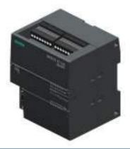
SIMATIC S7-200 SMART CPU CR20s, COMPACT CPU, AC/DC/RELAY, ONBOARD I/O: 12 DI 24V DC; 8 DO RELAY 2A; POWER SUPPLY: AC, 85 - 264 V AC AT 47 - 63 HZ, PROGRAM/DATA MEMORY: 20 KB
