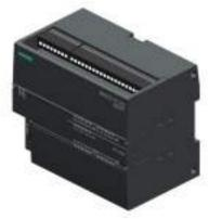
SIMATIC S7-200 SMART CPU CR40s, COMPACT CPU, AC/DC/RELAY, ONBOARD I/O: 24 DI 24V DC; 16DO RELAY 2A; POWER SUPPLY: AC, 85 - 264 V AC AT 47 - 63 HZ, PROGRAM/DATA MEMORY: 20 KB
